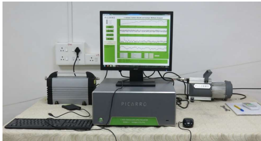
Figure 2: The Picarro greenhouse gas analyzer. It measures \text{CO}_2 and \text{CH}_4 concentrations, and their carbon isotopic ratios.
