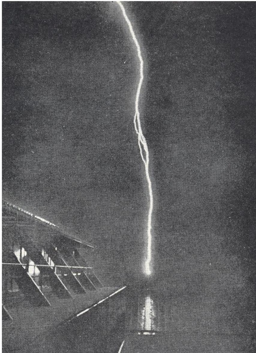
Lightning stroke to chimney pot showing meeting point between downward leader and upward streamer.
