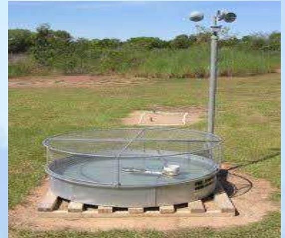
An atmometer or evaporimeter is a scientific instrument used for measuring the rate of water evaporation from a wet surface to the atmosphere.
