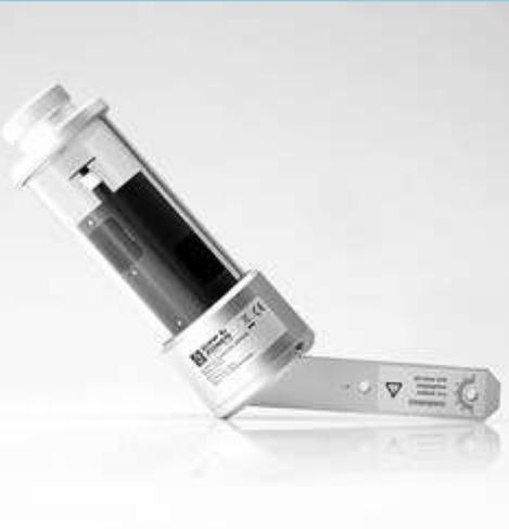
CSD3 measures sunshine duration. Sunshine duration is defined by WMO as the time during which the direct solar radiation exceeds the level of  $120 \text{ W/m}^2$ .
