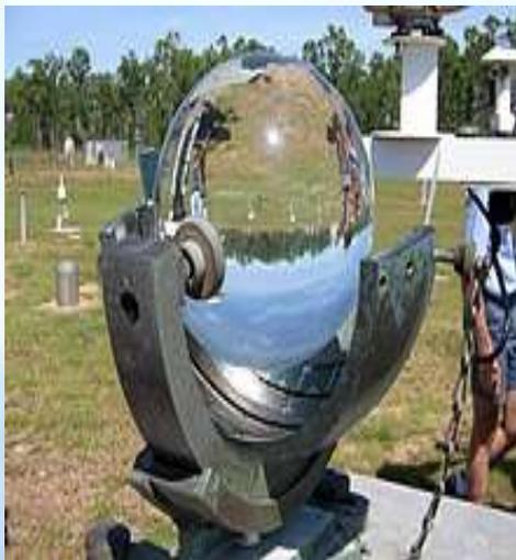
Measurement is performed by instruments called sunshine recorders. For the specific purpose of sunshine duration recording, Campbell–Stokes recorders are used, which use a spherical glass lens to focus the sun rays on a specially designed tape. When the intensity exceeds a pre-determined threshold, the tape burns.
