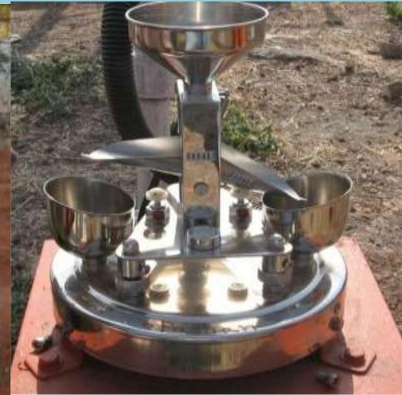
The sensor is the tipping bucket mechanism and is mounted at a height of 0.6 to 1 m. The collector diameter is 20 cm.
