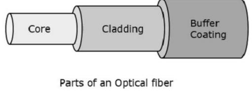
A solid di-electric material surrounds the core, which is called as Cladding. Cladding has a refractive index n2 which is less than n1. Cladding reflects the light back into the core. Cladding helps in –
