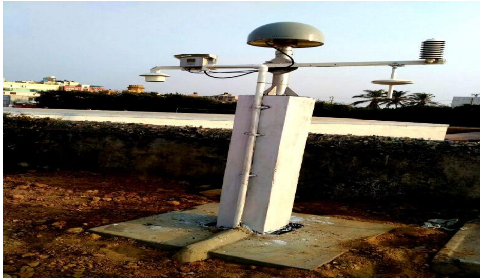
Fig. Vaisala Meteorological Sensor Co-located with GNSS Antenna. Station - Delhi.
