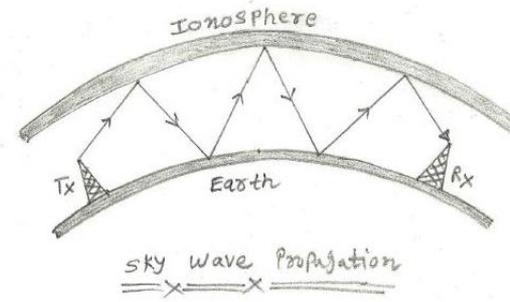
1. **Sky wave propagation** (suitable bandwidth for this type of communication is broadly between 2–30 MHz and makes use of the ionosphere properties of the earth) ex-MOBILE COMMUNICATION
