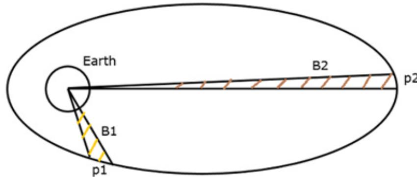
Assume, the satellite covers p1 and p2 distances in the same time interval. Then, the areas B1 and B2 covered by the satellite at those two instances are equal.
