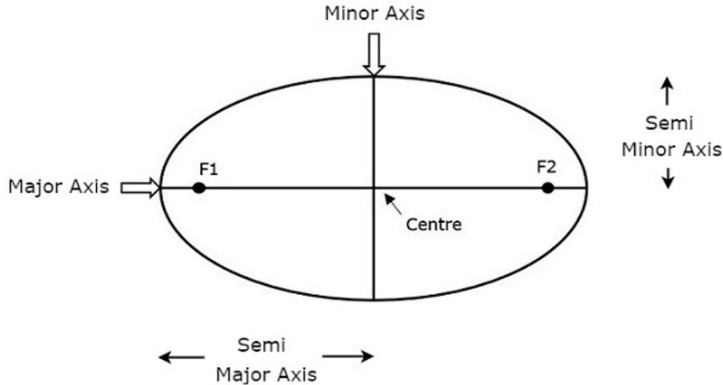
Both semi major axis and semi minor axis are represented in above figure. Length of semi **major axis (a)** not only determines the size of satellite's orbit, but also the time period of revolution.
