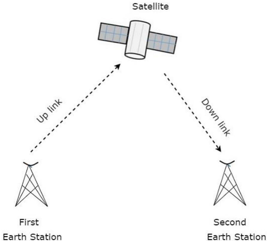
The transmission of signal from first earth station to satellite through a channel is called as uplink. Similarly, the transmission of signal from satellite to second earth station through a channel is called as downlink.
