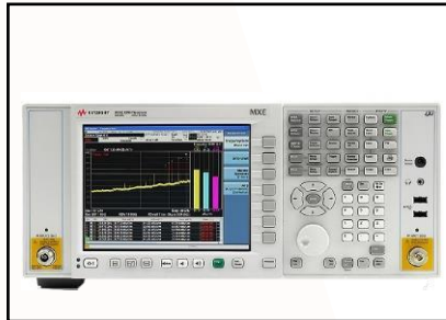
EMI Receiver Frequency : 3 Hz to 44 GHz Input Power: +30 dBm
