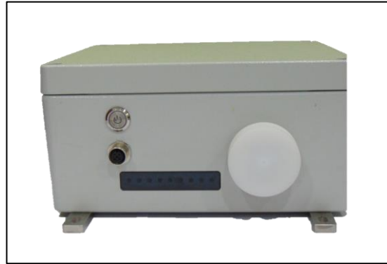
RADIOSONDE GROUND SYSTEM (ASAC-5750)
