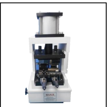
IC Forming & Cutting Forming Rate : 1000 parts/Hr
