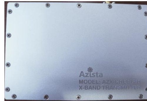
X-BAND TM TRANSMITTER 1 GBPS data
