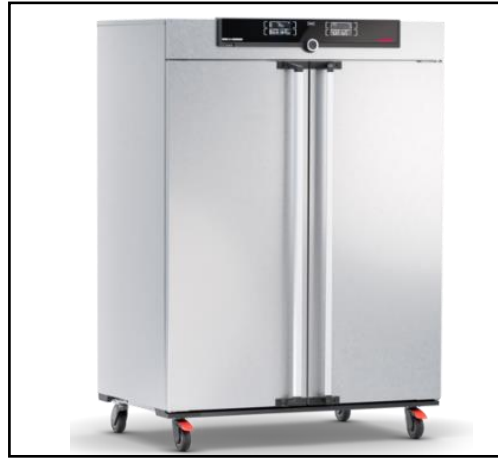
Environmental chamber Temp. Range: +5°C to 70°C Humidity Range: 10% to 90%
