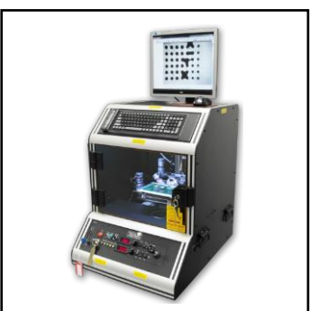
X-ray testing FoV: 25mm Magnification : 7x - 500x
