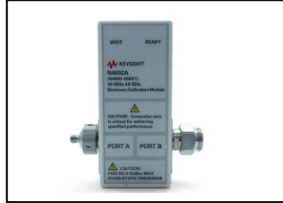
Electronic Calibration Module Frequency: 18 MHz to 40 GHz
