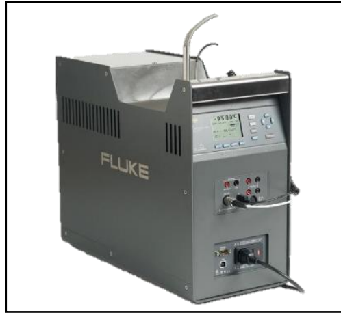
Field Metrology Well Temperature : -95°C to +140°C Accuracy : \pm 0.2 °C
