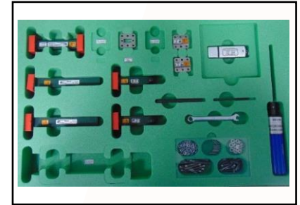
Waveguide Calibration Kit Frequency : 3.2 to 40.0 GHz
