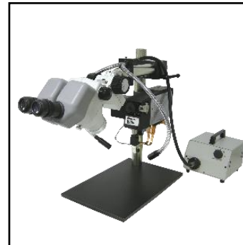
Ribbon Bonder Au Ribbon: 1 mil, 5 mil, 10 mil, 20 mil
