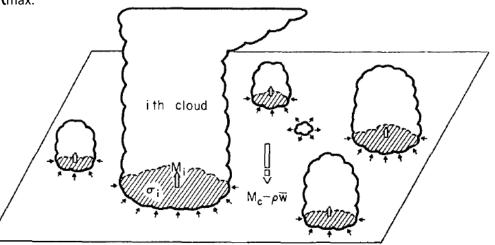
A unit horizontal area at some level between cloud base and the highest cloud top. The taller clouds are shown penetrating this level and entraining environmental air. A cloud which has lost buoyancy is shown detraining cloud air into the environment.
