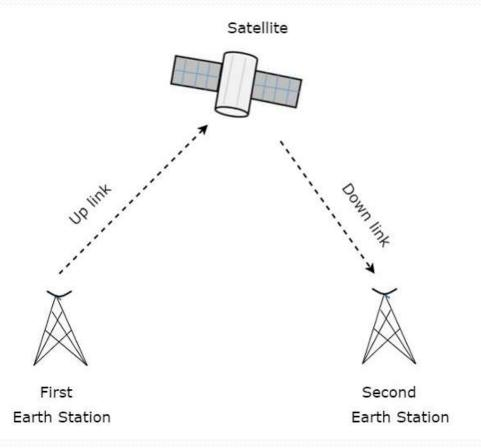
The transmission of signal from first earth station to satellite through a channel is called as uplink. Similarly, the transmission of signal from satellite to second earth station through a channel is called as downlink.
