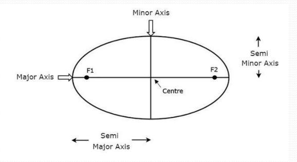
Both semi major axis and semi minor axis are represented in above figure. Length of semi **major axis** (a) not only determines the size of satellite's orbit, but also the time period of revolution.
