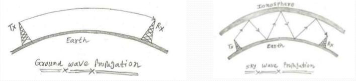
1. Sky wave propagation (suitable bandwidth for this type of communication is broadly between 2–30 MHz and makes use of the ionosphere properties of the earth) ex-MOBILE COMMUNICATION
