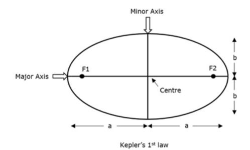
If the distance from the center of the object to a point on its elliptical path is considered, then the farthest point of an ellipse from the center is called as **apogee** and the shortest point of an ellipse from the center is called as **perigee**.
