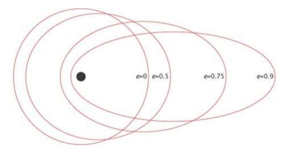
In above figure, the satellite orbit corresponding to eccentricity (e) value of zero is a circular orbit. And, the remaining three satellite orbits are of elliptical corresponding to the eccentricity (e) values 0.5, 0.75 and 0.9.
