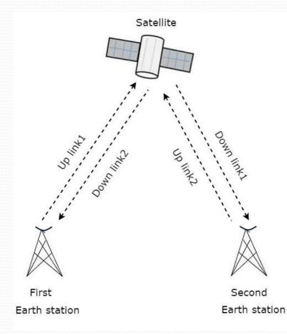
Here, the communication takes place between first earth station (transmitter) and second earth station (receiver) on earth's surface through a satellite in **two** (both) **directions**.
