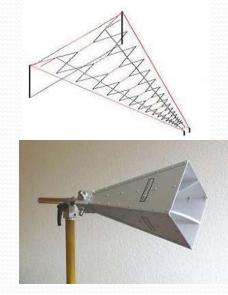
Horn antennas are used in **microwave** frequency range. The same feed horn can be used for both transmitting and receiving the signals. A device named **duplexer**, which separates these two signals.
