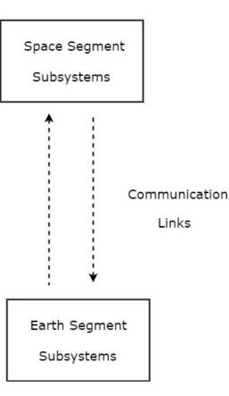
As shown in the figure, the **communication** takes place between space segment subsystems and earth segment subsystems through communication links.
