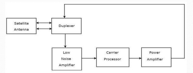
•Duplexer is a two-way microwave gate. It receives uplink signal from the satellite antenna and transmits downlink signal to the satellite antenna.
