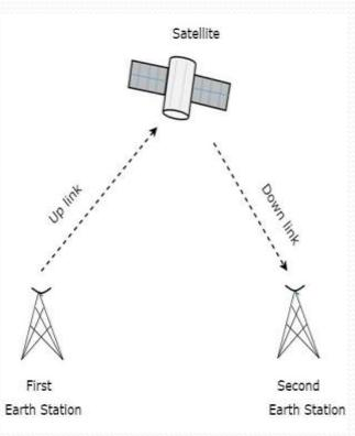
Here, the communication takes place between first earth station (transmitter) and second earth station (receiver) on earth's surface through a satellite in **one direction**.
