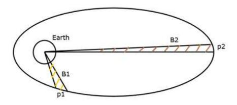
Assume, the satellite covers p1 and p2 distances in the same time interval. Then, the areas B1 and B2 covered by the satellite at those two instances are equal.
